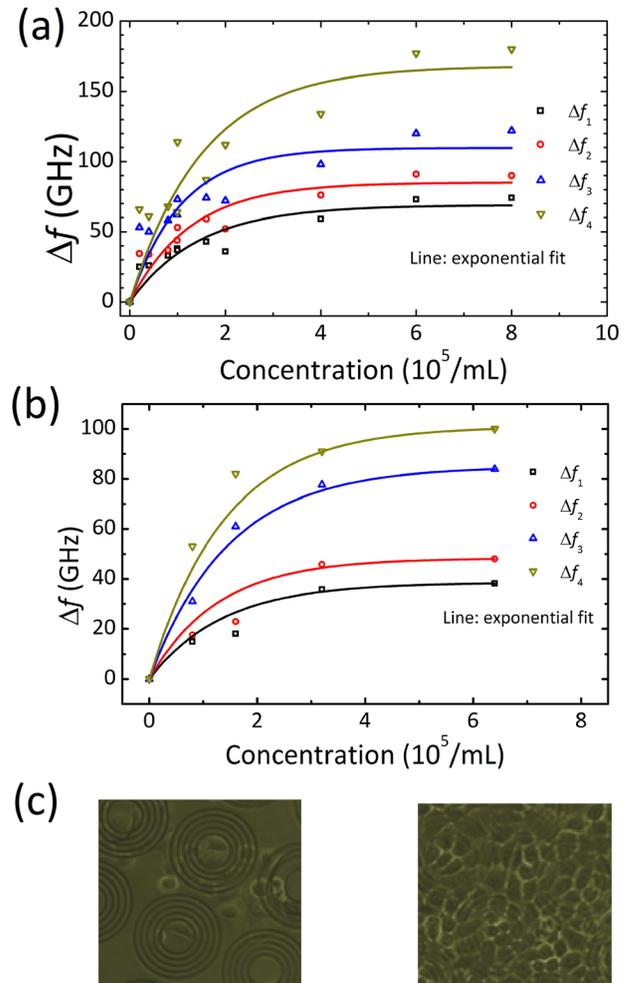
FIG. 2. The frequency shift  $\Delta f$  of metamaterial with and without cell analyte versus concentration for tumor cell (HSC3) (a) and normal cell (HaCaT) (b); symbols are experimental results and lines are exponential fit. (c) Micrograph of our biosensor with cell analyte HSC3 at a concentration of  $2 \times 10^5$  cells/ml (left) and  $6 \times 10^5$  cells/ml (right).
