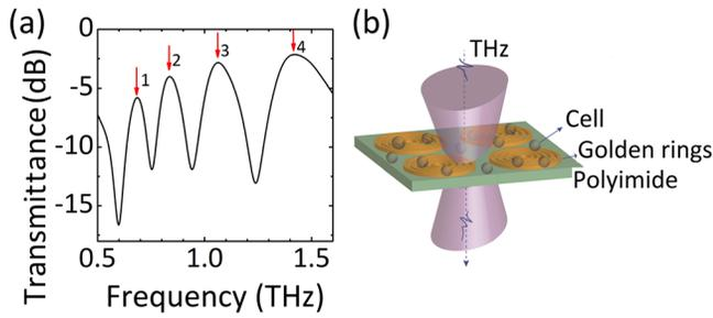
FIG. 1. (a) The transmission spectra of bare metamaterial; (b) The schematic diagram of THz TDS measurement. The unit cell of metamaterial has a period of  $120\ \mu\text{m}$ , and the inner radius of five rings is  $20\ \mu\text{m}$ ,  $28\ \mu\text{m}$ ,  $36\ \mu\text{m}$ ,  $44\ \mu\text{m}$ , and  $52\ \mu\text{m}$ , respectively. The linewidth of each ring and the distance between adjacent rings both have a size of  $4\ \mu\text{m}$ .
