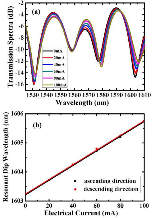
**Fig. 3.** (a) Transmission spectra of the sensor under different electrical current when 75 mT magnetic field is applied. (b) Relationship between the resonant dip wavelength and electrical current in ascending and descending directions.
