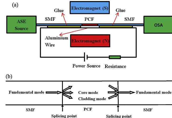
**Fig. 1.** (a) Schematic diagram of the experimental setup used for magnetic field sensing measurement. (b) Schematic diagram of the modal interference of the PCFMI.
