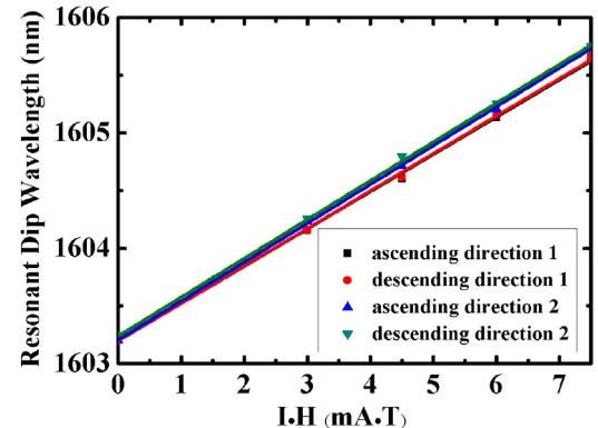
**Fig. 4.** Relationship between the resonant dip wavelength and  $I \cdot H$  in ascending and descending directions.
