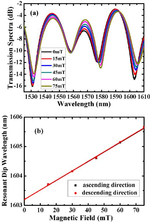
**Fig. 2.** (a) Transmission spectra of the sensor under different magnetic field when 100 mA electrical current is applied. (b) Relationship between the resonant dip wavelength and magnetic field in ascending and descending directions.
