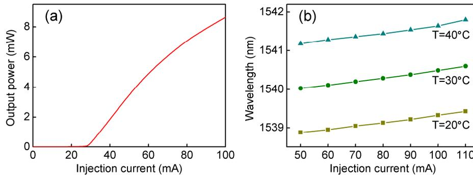
Fig. 3. (a). Light-current characteristic of the REC based DFB laser; (b) lasing wavelengths at different injection currents (above threshold) and temperatures.
