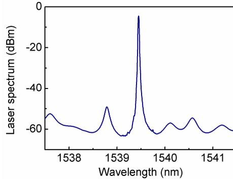
Fig. 2. Typical laser spectrum of the REC based DFB laser at the injection current of 40mA.
