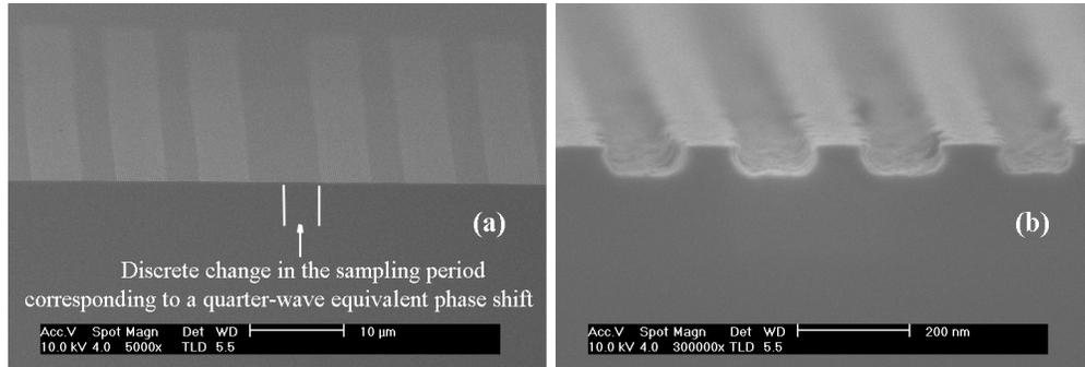
Fig. 1. Illustration of the SEM morphology of: (a) sampled grating with a quarter-wave equivalent phase shift; (b) uniform Bragg gratings in a sampling period.
