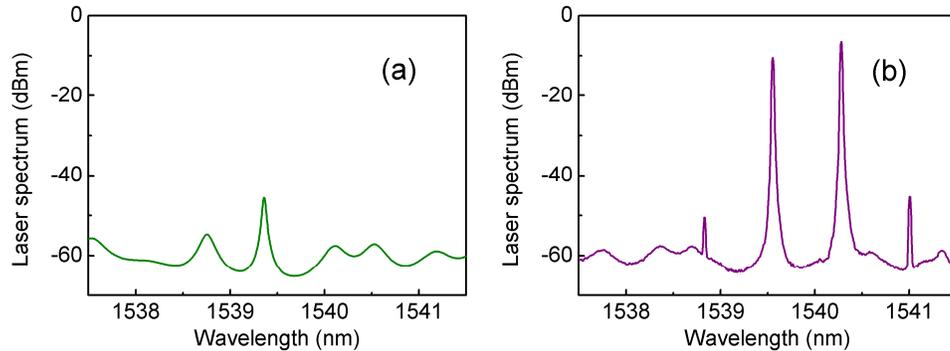
Fig. 4. Typical laser spectra at the injection currents of 27mA (a) and 100mA (b).
