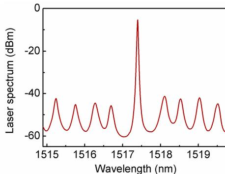
Fig. 6. REC based DFB semiconductor laser with a different wavelength in a different part of the same chip at the injection current of 20mA.
