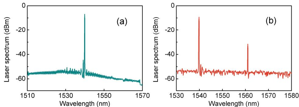
Fig. 5. Typical laser spectra of the REC based DFB laser in a wide wavelength range at the injection currents of 70mA (a) and 140mA (b).
