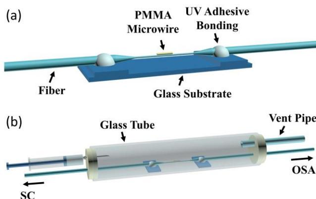
Fig. 1. Schematic diagram of (a) hybrid microfiber coupler and (b) experimental device; SC, supercontinuum; OSA, optical spectrum analyzer
