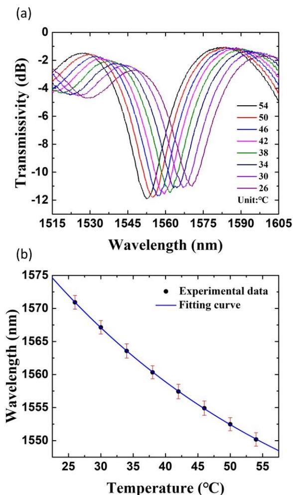
Fig. 5. Resonant wavelength shift as a function of temperature. The sensitivity at room temperature was approximately  $-942 \text{ pm}/^\circ\text{C}$ .
