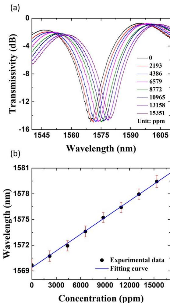
Fig. 4. (a) Transmission spectra with different concentrations of ethanol vapor. (b) Resonant wavelength shift as a function of the vapor concentration. The sensitivity was approximately 0.65 pm/ppm.
