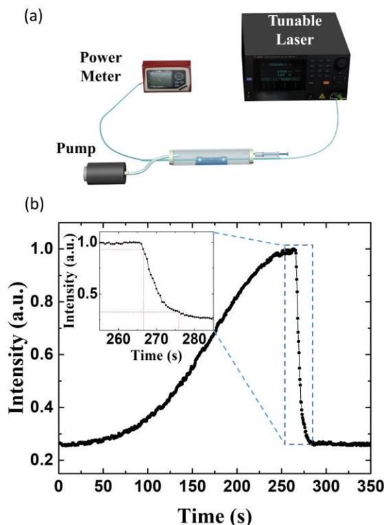
Fig. 6. (a) Experimental setup to measure the dynamic response. (b) Time response of the coupler. Inset shows that the recovery time was 9.4 s.
