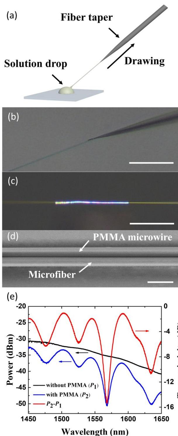
Fig. 2. (a) Fabrication of a PMMA microwire; (b) PMMA microwire picked up using a fiber probe; (c) micrograph, (d) SEM, and (e) output spectrum of the hybrid microfiber coupler. Scale bar: (b) (c) 100  $\mu\text{m}$ , (d) 2  $\mu\text{m}$
