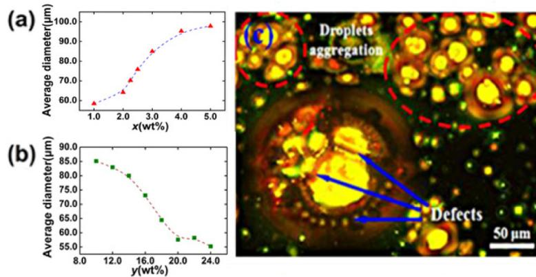
Fig. 3. Average diameter of CLC micro-droplets changes with the increasing of (a) CLC concentration when PVA concentration is 18.0 wt%; and (b) PVA concentration when CLC concentration is 2.0 wt%. (c) Texture micrograph of CLC droplets in the case of  $x = 4.0$  wt% and  $y = 14.0$  wt%.
