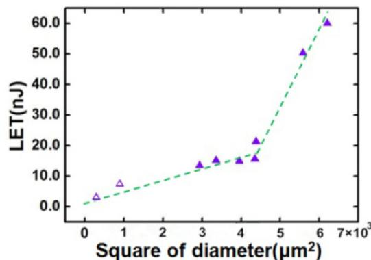
Fig. 4. Relationship between LET and the square of diameter of CLC micro-droplet. Hollow triangles indicate that the probability of the lasing of smaller droplet is lower than that of larger ones.
