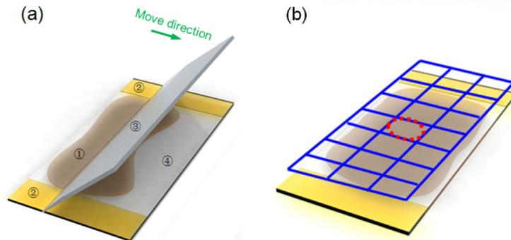
Fig. 1. Schematics of (a) the preparation of CLC micro-droplet laser (①:emulsion ②:Kapton strip ③:doctor blade ④:glass substrate); (b) numerical statistic of effective CLC micro-droplets (the whole sample was divided into twenty-one square regions as depicted by blue solid cross-lines; number of effective droplets in every square region as enclosed by red dashed circle was counted one by one and summed up).
