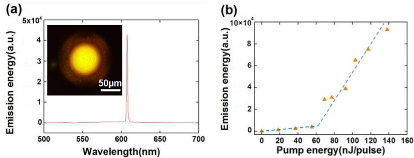
Fig. 2. (a) Emission spectrum of a CLC micro-droplet and the corresponding optical texture (the inset) and (b) the pump energy dependent lasing emission energy of such micro-droplet. Concentrations of CLC and PVA are 2.0 wt% and 18.0 wt%, respectively. Diameter of the focused pumping light is manipulated to approximately equal to the diameter of the micro-droplet, which is  $\sim 120 \mu\text{m}$ , and the repetition rate of pumping light is 1 Hz.
