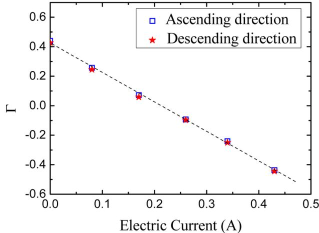
Fig. 6.  $\Gamma$  dependence on electric current in the wavelength of 1543 nm under 2 mT perpendicular magnetic fields in ascending and descending directions. The curve represents the linear fitting of the data.
