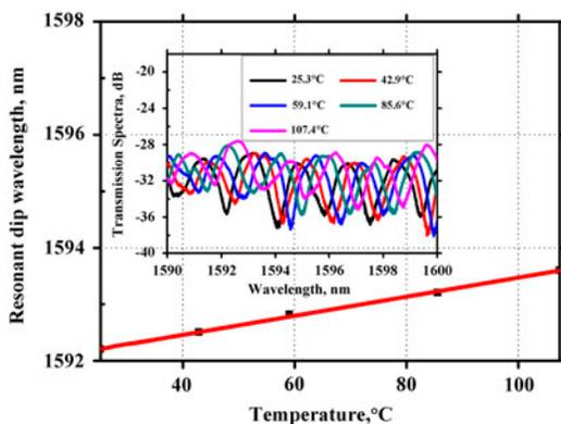
Figure 3. Relationship between temperature and the resonant dip wavelength. The inset shows the transmission spectra of the SGF interferometer under different temperatures. (The color version of this figure is included in the online version of the journal.)
