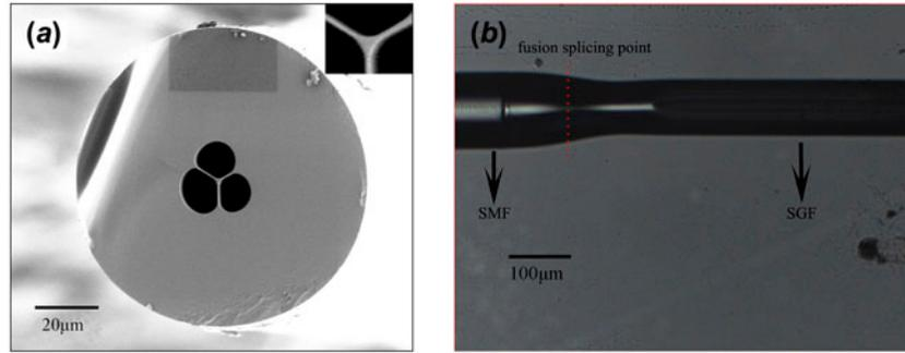
Figure 1. (a) Scanning electron microscope image of the cross-section of the SGF. The insert is a magnification of the core of the SGF. (b) Microscopic image of the fiber fusion splicing area showing the collapsed region at the end of the SGF. The dotted line denotes the fusion splicing point. (The color version of this figure is included in the online version of the journal.)
