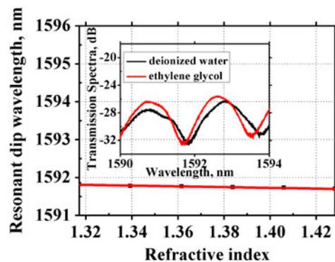
Figure 4. Relationship between outer liquid RI and the resonant dip wavelength. The inset shows the transmission spectra of the SGF interferometer when immersed in different liquids. (The color version of this figure is included in the online version of the journal.)
