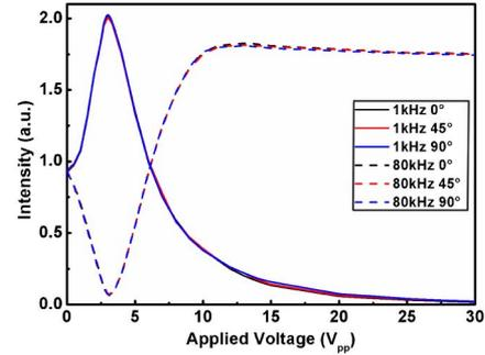
Fig. 4. (Color online) Voltage dependent intensities of first order at 1 kHz and 80 kHz when the sample is placed at three different directions: 0, 45, and 90 deg relative to the incident polarization.
