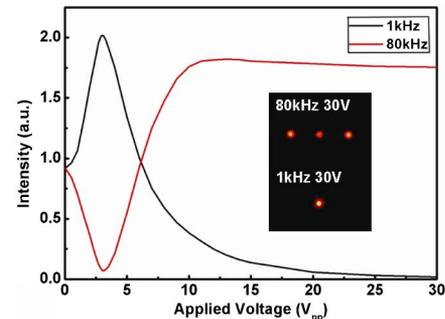
Fig. 2. (Color online) Voltage dependent intensities of first order at 1 kHz and 80 kHz. Insets show diffraction patterns at the On and Off states.
