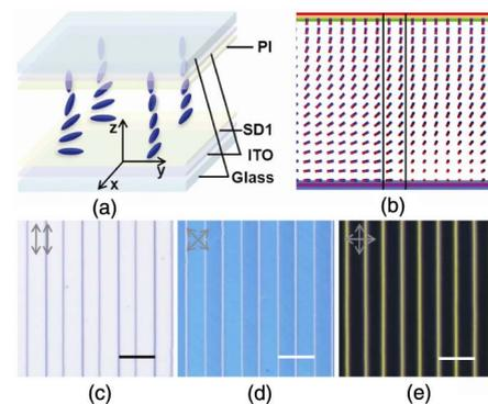
Fig. 1. (Color online) (a) Schematic illustration of the patterned HAN cell; (b) LC director distribution in  $y$ - $z$  plane simulated by Techviz LCD with two black lines marking the boundary region, and (c)–(e) micrographs of the sample, in each of which the relative directions of two polarizers compared with the stripes are labeled in arrows. All scale bars are 20  $\mu\text{m}$ .
