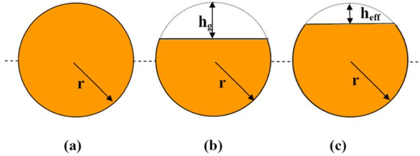
Fig. 2. The cross-sections of (a) an un-etched fiber, (b) an etched fiber and (c) an equivalent unperturbed geometry, respectively.  $h_g$  is the groove height and  $h_{\text{eff}}$  is effective height.
