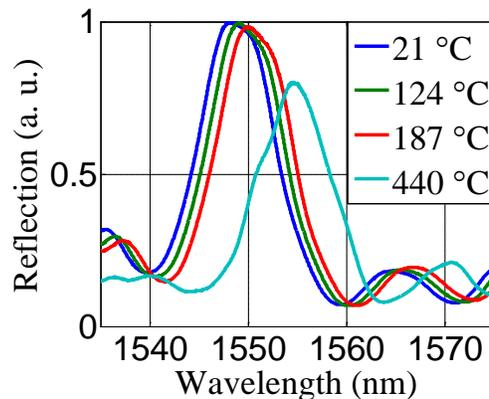
Fig. 3. Reflection spectra of the TFPG in air at different temperatures.
