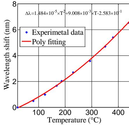
Fig. 4. Dependence of the measured wavelength shift on temperature. The asterisk represents the measured results while the solid line is the linear fitting result.
