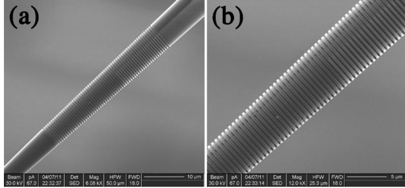
Fig. 1. (a) FIB picture of the TFPG with 61 periods ( $\sim 36.6 \mu\text{m}$  in length and  $\Lambda = 600$  nm). (b) Magnified picture of the grating.
