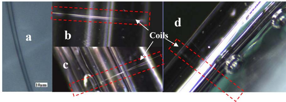
Fig. 2. Microscope pictures of a MCR (a) wrapped on a rod (b), (c) before and (d) after embedded in Teflon. (b) and (c) are taken from different sides. The microfiber and rod radii are  $\sim 1.5$  and  $500\mu\text{m}$ , respectively.
