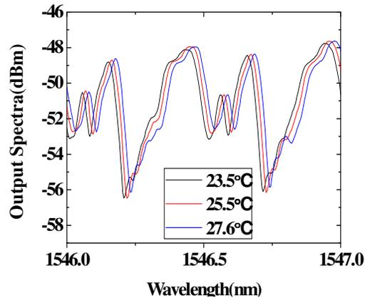
Fig. 4. Transmission spectra of the embedded MCR at three different temperatures.
