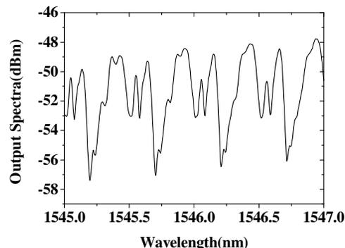
Fig. 3. Transmission spectrum of the embedded MCR onto a 1-mm-diameter support rod in the range from 1545 to 1547 nm.
