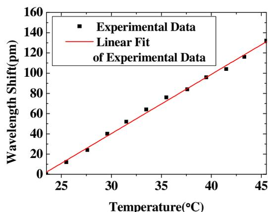
Fig. 5. Variation of the resonance wavelength in the embedded MCR as a function of temperature.
