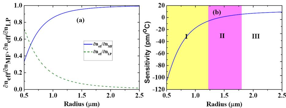
Fig. 1. (a) Variation of  $\partial n_{eff}/\partial n_{MF}$  (solid line) and  $\partial n_{eff}/\partial n_{LP}$  (dashed line) as a function of the microfiber radius. (b) Variation of the estimated sensitivity as a function of the microfiber radius, only considering the contribution from thermo-optic effect. Red area II is the temperature insensitive area where  $|S| < 5\text{pm}/^\circ\text{C}$ .
