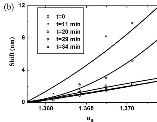
Fig. 3. (a) Interference spectra of the tapered PCF interferometers in air. (b) Wavelength shifts due to surrounding refractive index changes before and after the interferometer was etched by a small HF microdroplet. Here, the etching time  $t$  is the total time accumulated by all these tapering periods before the spectra were measured.
