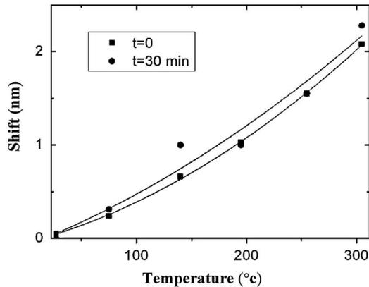
Fig. 4. Wavelength shifts due to temperature change before and after the interferometer was etched by HF microdroplets.
