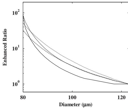
Fig. 2. Enhanced ratios for several cladding modes as a function of the diameter of a tapered PCF.
