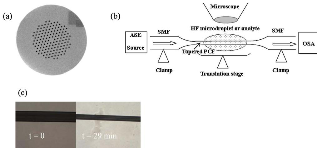
Fig. 1. (Color online) (a) Scanning electron microscope image of the cross section of the PCF used for the experiment. (b) Schematic of the experimental setup for tapering and sensing measurement. The PCF length is  $L$  and the diameter of the tapered PCF is  $D$ . OSA, optical spectrum analyzer. (c) Pictures of the PCF before etching and after 29 min of etching.
